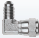
COMPACT ELBOW 90° – FORGED JIC MALE / JIC SWIVEL FEMALE
