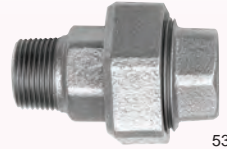
UNION TAPER SEAT BSPT MALE / BSPP FEMALE
